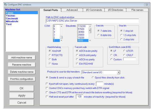
Click ADD MACHINE NAME and enter appropriate settings for your machine control. Always copy config from another machine so that the basic defaults are set properly, then modify settings for specific machine using the information on the link below for CNC configs. Repeat for additional machines. To get assistance with parameters for common CNC controls, visit
